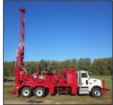
Most well drilling rigs are over the legal road limit for both gross and axle weights, based on their configurations. This is due to the tools and equipment that they are set up for in order to perform the job they are designed to do. As such, the vehicles cannot be registered in the same manner as trucks or truck tractors and must be registered as **Special Mobile Equipment, Class A**.
